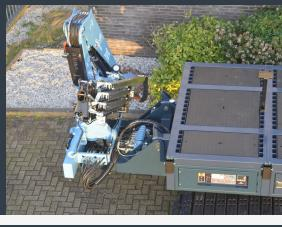
Versatile Crane Booms, by means of two knuckle booms, Crane Boom rotation and impressive Telescopic boom. Fully proportional controlled and each Crane function operated by a dedicated joystick controller.
